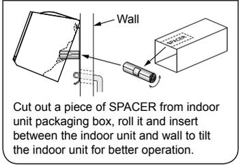
Cut out a piece of SPACER from indoor unit packaging box, roll it and insert between the indoor unit and wall to tilt the indoor unit for better operation.
