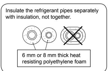
Insulate the refrigerant pipes separately with insulation, not together.
