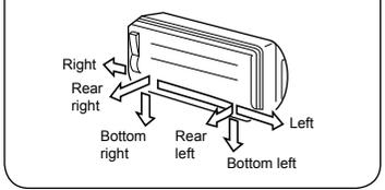
The auxiliary piping can be connected to the left, rear left, rear right, right, bottom right or bottom left.
