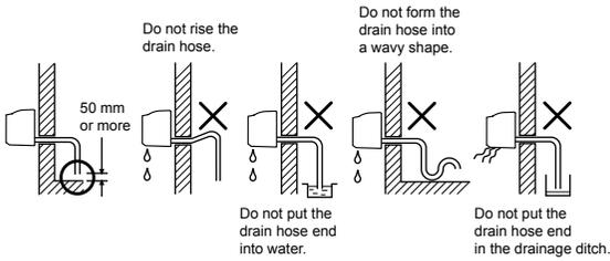
2. Put water in the drain pan and make sure that the water is drained out of doors.
