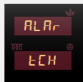
Alarm Thermocouple in the Chamber
